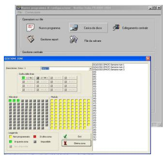
The programming functions that can be realized by using this software are the same the user can carry out working on the control panel. PK software is Windows XP compatible. The communication between control panel and PC is realized through RS232 serial port.
